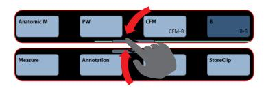
Activate/deactivate measurement controls by pressing "Measure" after freezing the image.
