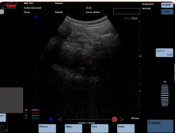
Place the first grey caliper with the touchpad in the desired place to start to measure the distance D1. Press Set. The second caliper is now displayed. Place it with the touch pad and click Valid to validate the measurement.
