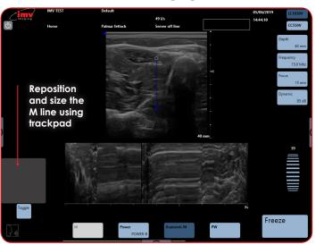
Place the start of the Anatomic M line with the trackpad, then press Toggle in order to position the arrow that symbolizes the end of the Anatomic M line specter.
